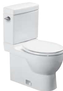
TWIST 5C11 01 Round-front 12" rough-in 1.28 gpf, siphonic jet 5D07 U1 Tank 9M08 U1 seat & cover with quick release & soft-closing hinges
