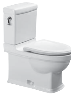
STRADA 5C14 01 Elongated 12" rough-in 1.28 gpf, siphonic jet 5D06 U1 Tank 9M04 S1 seat & cover with quick-release & soft closing hinges
