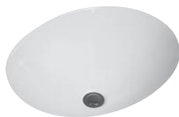
ARCHITECTURA 5A19 19 19" x 15 1/4" 5A19 17 17" x 14" 5A19 15 15" x 12 1/4" Oval shape Interior glazed only Centered drain, with overflow
