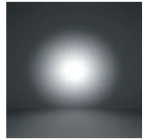
WF - Wide Flood α from 40° to 60°
