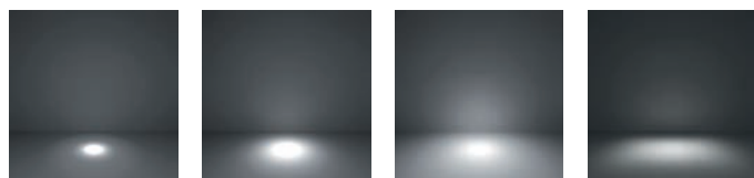
S - Spot α from 9° to 15° M - Medium α from 16° to 25° F - Flood α from 26° to 39° E - Elliptical*
