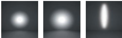
F - Flood \alpha from 26° to 39° WF - Wide Flood \alpha from 40° to 60° E - Elliptical*
