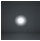
S - Spot \alpha from 9^\circ to 15^\circ
