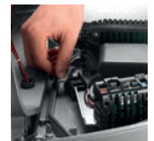
Tool-free replacement of power supply
