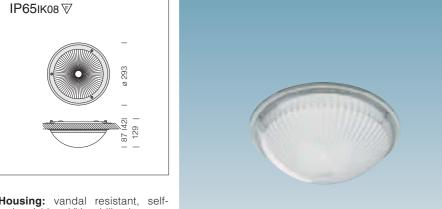
**Housing:** vandal resistant, self-extinguishing, UV-stabilised. **Diffuser:** vandal resistant, V2 self-extinguishing, UV-stabilised clear polycarbonate, anti-glare matt inside; smooth, dust-proof outside. LED: Power factor >0.9
