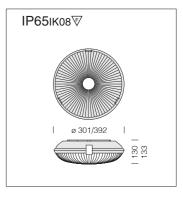
**Housing:** vandal resistant, selfextinguishing, UV-stabilised. **Diffuser:** vandal resistant, V2 selfextinguishing, UV-stabilised clear polycarbonate, anti-glare matt inside; smooth, dust-proof outside. **LED:** Power factor >0.9
