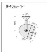
Housing: Die-cast aluminium with accessible frame designed with bayonet coupling to allow easy lamp maintenance.
