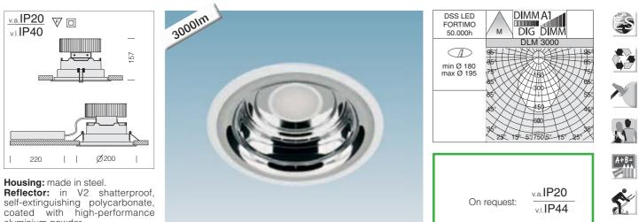
aluminium powder. LED: Luminous flux maintenance L70B50: 50.000h.
