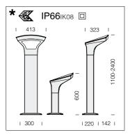
Housing/Base: in die-cast aluminium. Column: in extruded aluminium.
