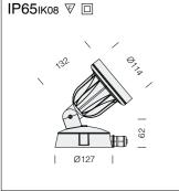
Housing/frame: in die-cast aluminium with wide cooling fins for heat dissipation.
