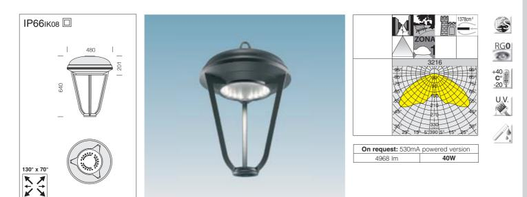
LED: Power factor ≥0.9. Luminous flux maintenance 70% 60000h (L70B20)
