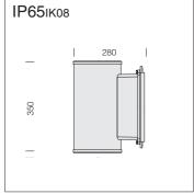
Housing: die-cast aluminium. Diffuser: tempered glass, 4 mm thick, shock and heat resistant LED: Luminous flux maintenance 70% 50000h (L70B50) Power factor ≥0.95
