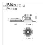
Housing: Adjustable angle, made of die-cast aluminium. **Reflector:** high-efficiency prismatic and polished aluminium. **LED:** Luminous flux maintenance L70B50: 50.000h. Power factor >0.9
