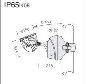
Housing: die-cast aluminium. Diffuser: tempered shock and heat resistant 4mm thick glass. LED: Luminous flux maintenance 70% 50000h (L70B50) Power factor ≥0.95
