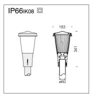
Housing/ Cap: in die-cast aluminium.
